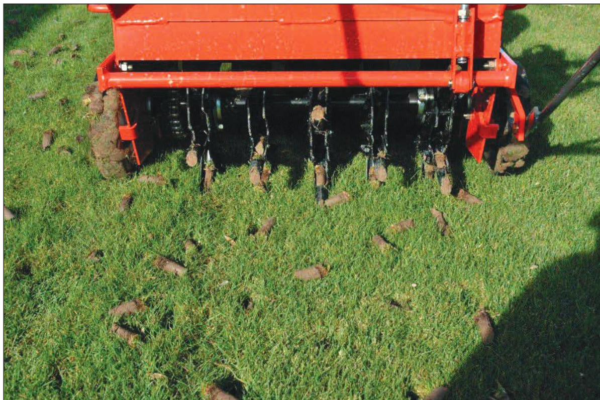
A plugging machine is used to removed spaced cores of thatch to aerate the lawn.
