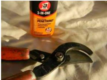
She was right. I put penetrating oil on the Pivot bolt and nut for three days. Absolutely no luck in loosening the bolt or nut using my standard socket set. In cases like this I find that I need to place the blade and the bolt and nut in a solvent.
