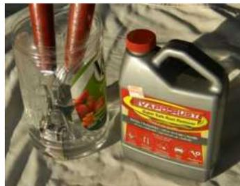
It helps to use #0 steel wool for cleaning the loppers. It's amazing how clean the loppers will be. With a funnel, pour the used rust remover back into its original container for another use. Place the loppers on your workbench, with the pivot nut facing up and spray the top of the nut with penetrating oil. Let stand for at least one day.
