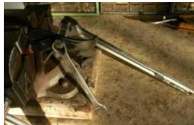
After the bolt and nut are removed, using a wire brush, clean the bolt and nut and the lopper blades as clean as you can. A bench grinder with a wire brush grinder is the best tool to use. Remember to wear your gloves, safety eye and ear protection devices. Note, the nut shows three notches where a wrench had slipped when someone was trying unsuccessfully to remove the pivot nut.
